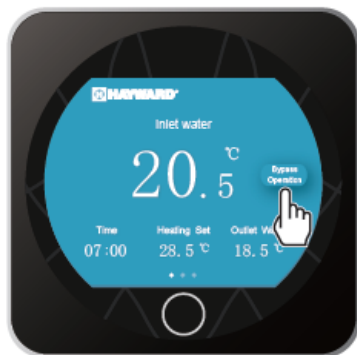
Activate Bypass Operation
