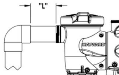
NOTE: It is recommended that a minimum length of straight piping (shown as “L” in above diagram), equivalent to 5 pipe size diameters, be used between the pump suction inlet and any plumbing fittings (elbows, valves, etc.).
