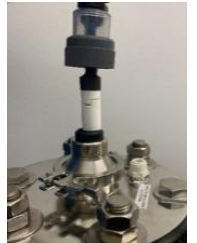
Quick-disconnect sleeve for easy maintenance
